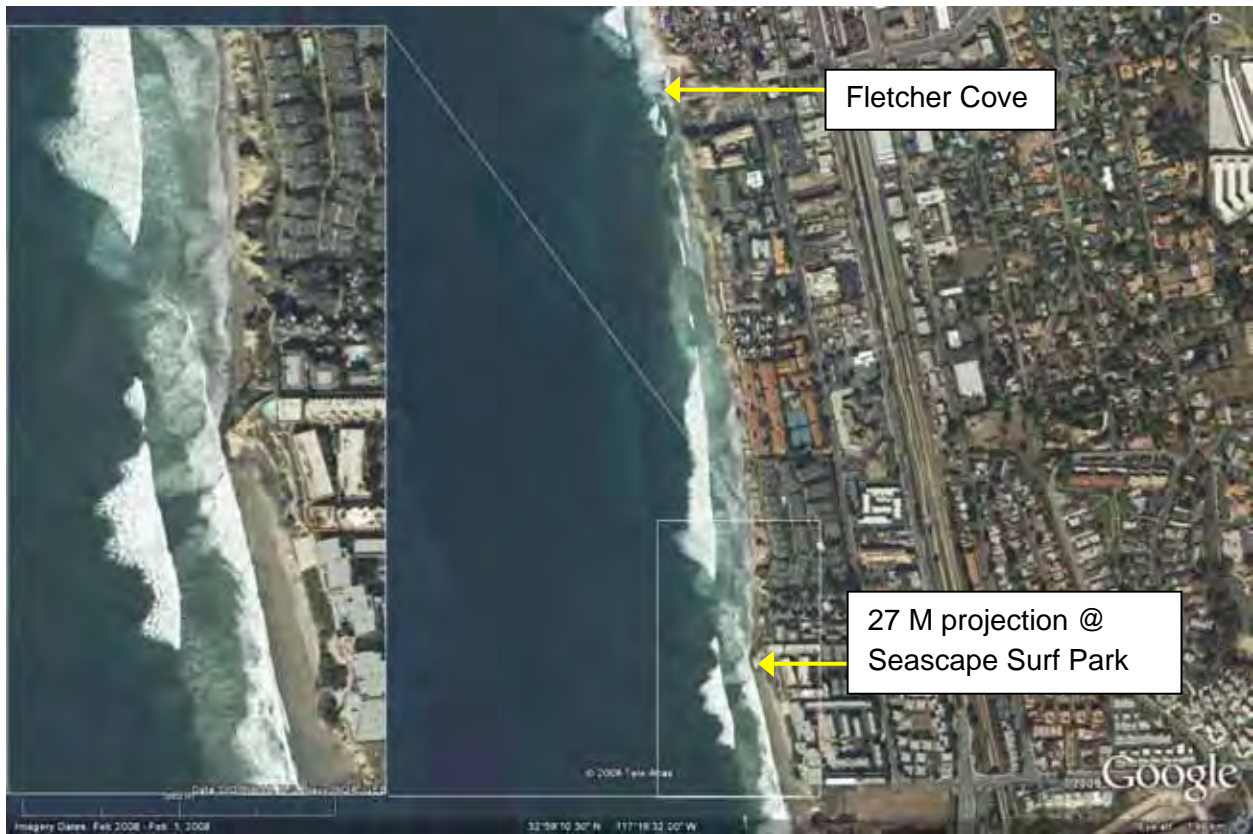
Figure 4.3 Longshore Transport Blocking Projection with no Fillet or Downcoast Erosion
